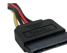
Serial ATA power connector
