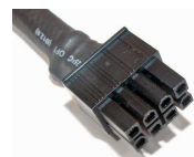
8-pin ATX 12 V
