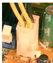
4-pin ATX 12 V
