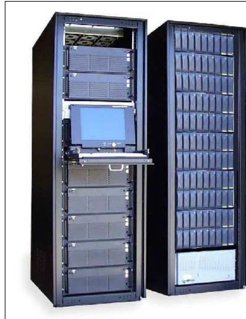
Early Aspen Systems Beowulf Cluster With RAID
