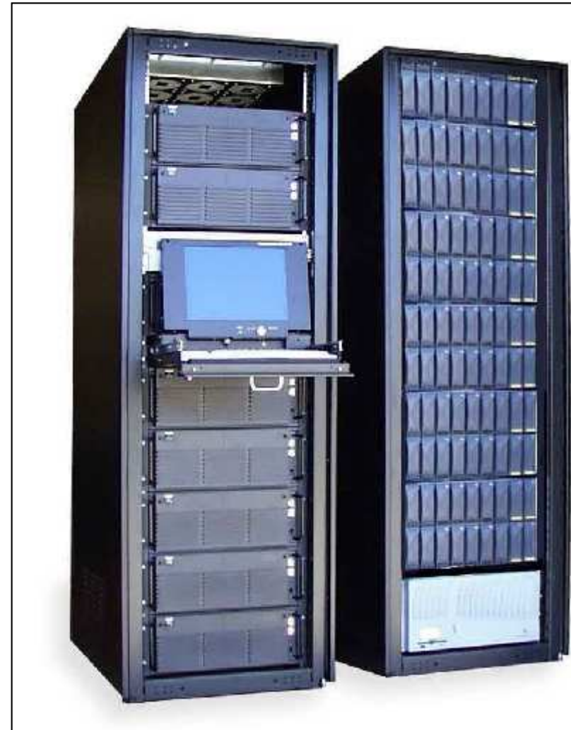
Early Aspen Systems Beowulf Cluster With RAID
