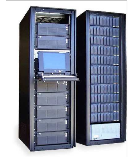
Early Aspen Systems Beowulf Cluster With RAID
