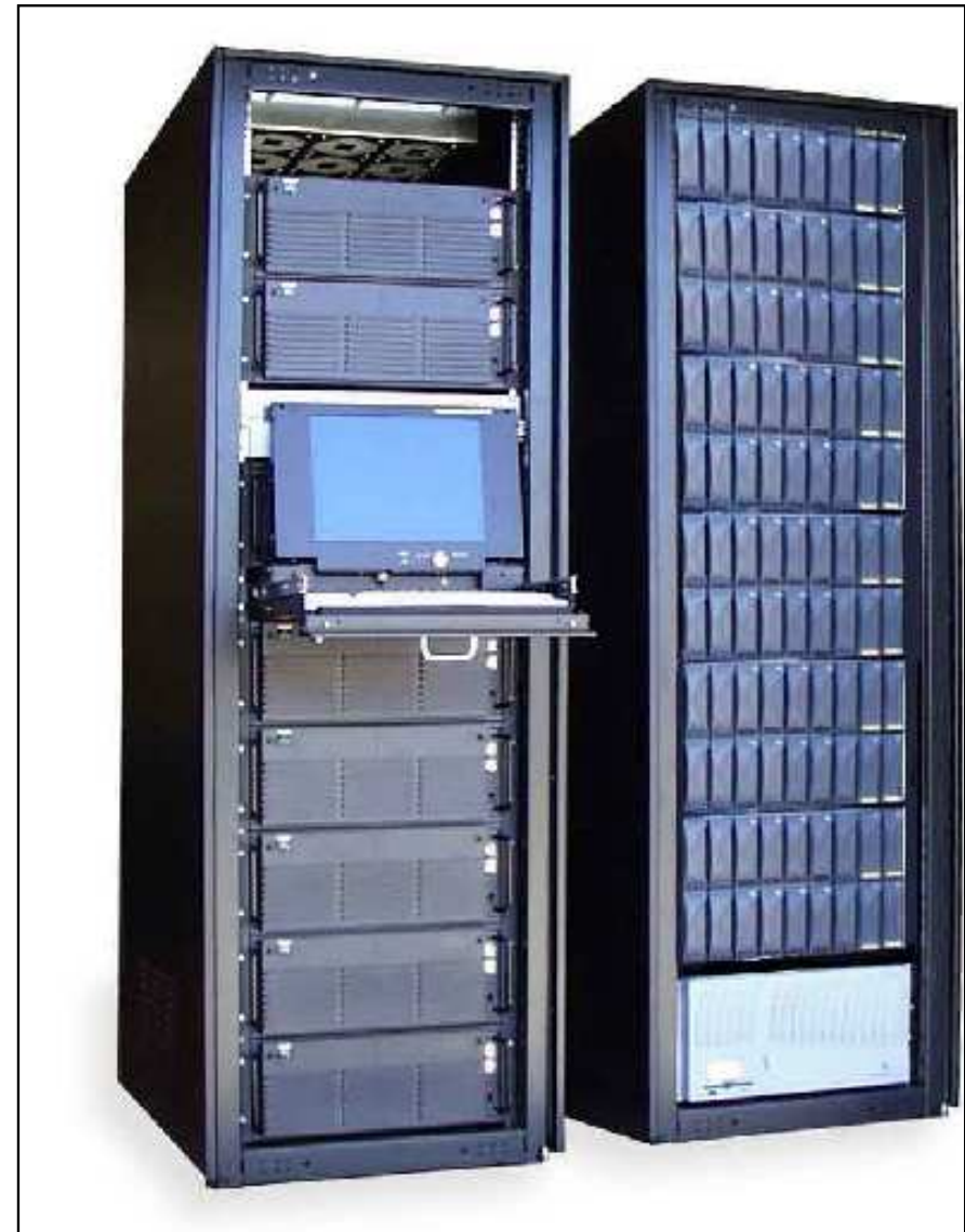
Early Aspen Systems Beowulf Cluster With RAID
