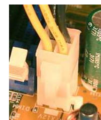
4-pin ATX 12 V
