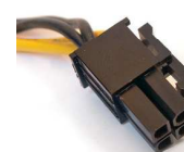
4-pin ATX 12 V
