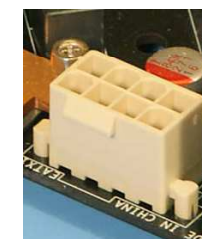
8-pin ATX 12 V
