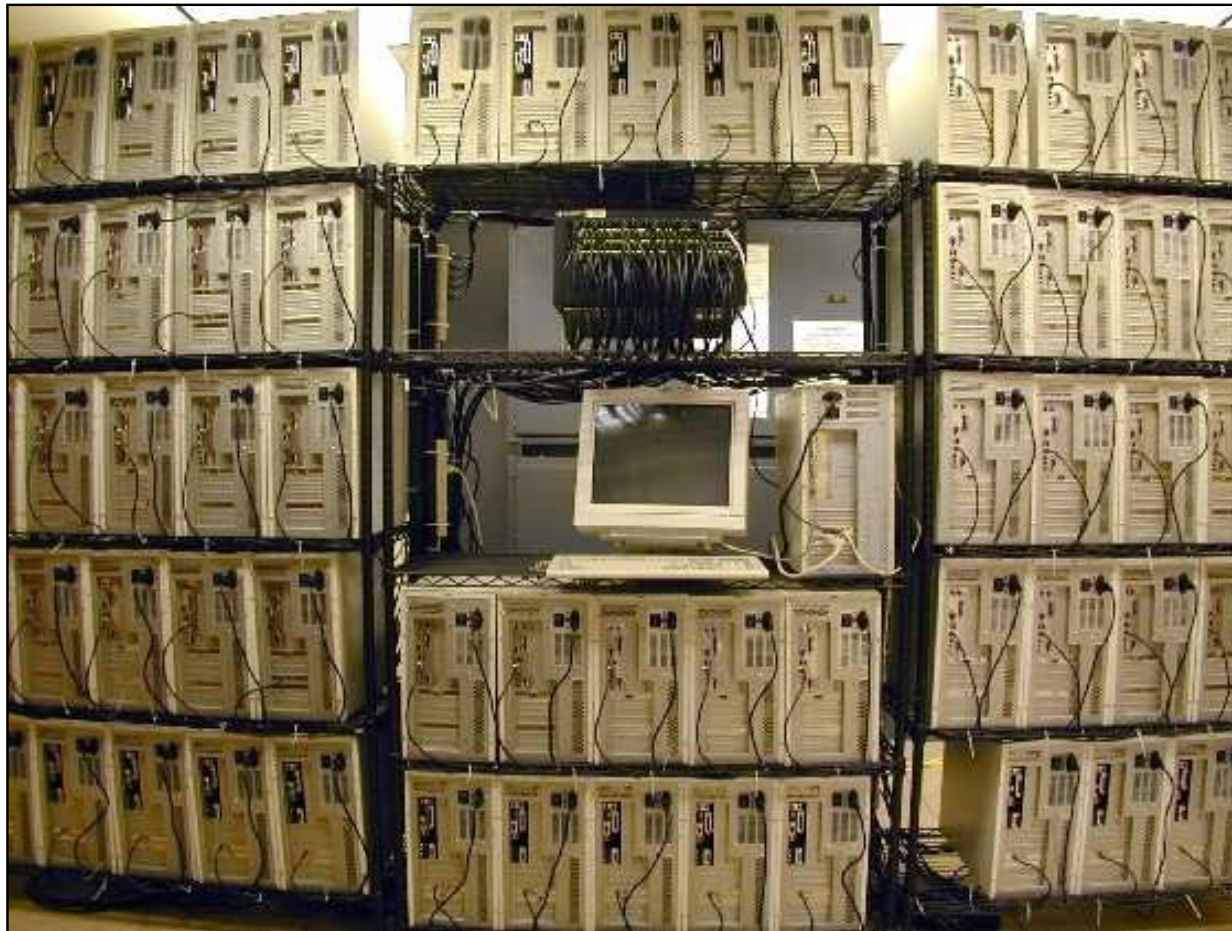
NASA 128-processor Beowulf cluster: A cluster built from 64 ordinary PC's
