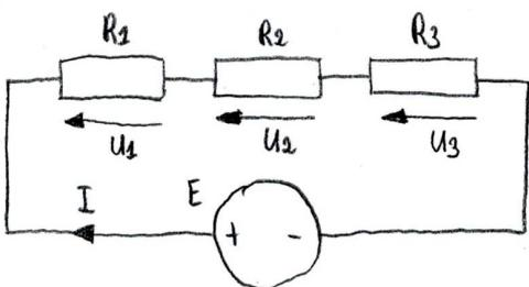
$$I = \frac{E}{R_1 + R_2 + R_3} = \frac{12}{1000 + 5000 + 10000} = \frac{12}{16000} = 0.75\text{ mA}$$
