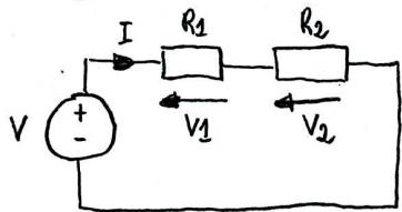
$$I = \frac{V}{R_1 + R_2} \quad V_1 = I \cdot R_1 \quad V_2 = I \cdot R_2 \quad R_1 \neq R_2 \rightarrow V_1 \neq V_2$$
