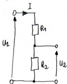
$$I = \frac{U_1}{R_1 + R_2} = \frac{100}{70 + 30} = \frac{100}{100} = 1 \text{ A}$$
