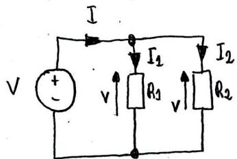
$$I_1 = \frac{V}{R_1} \quad I_2 = \frac{V}{R_2} \quad I = I_1 + I_2$$
