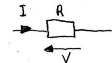
\* for given resistance, the current is directly proportional to voltage
