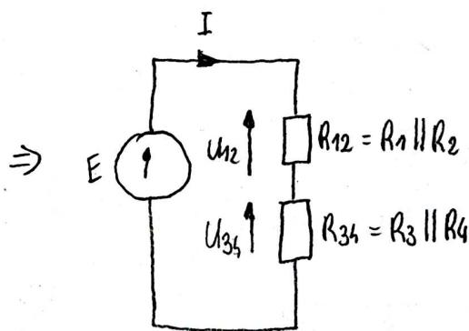
$$R_{12} = \frac{R_1 \cdot R_2}{R_1 + R_2} = \frac{10 \cdot 15}{10 + 15} = \frac{150}{25} = 6 \Omega$$
