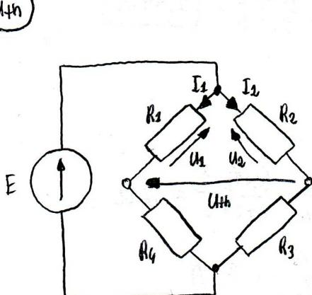
$$I_1 = \frac{E}{R_1 + R_4} = \frac{12}{4+4} = 1.5 \text{ A}$$
