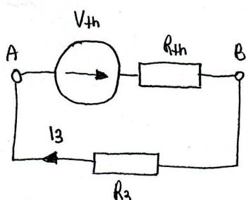
$$I_3 = \frac{V_{th}}{R_{th} + R_3} = 0$$
