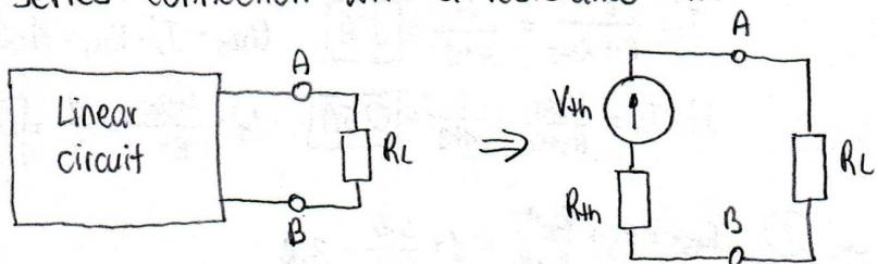
$V_{th}$  - the voltage obtained at terminals A-B of the circuit with terminals A-B open circuited
