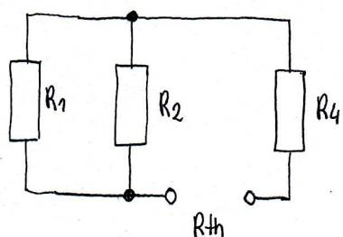
$$R_{th} = \frac{R_1 \cdot R_2}{R_1 + R_2} + R_4 = \frac{1 \cdot 2}{1+2} + 1 = \frac{2}{3} + 1 = \frac{5}{3} \Omega$$
