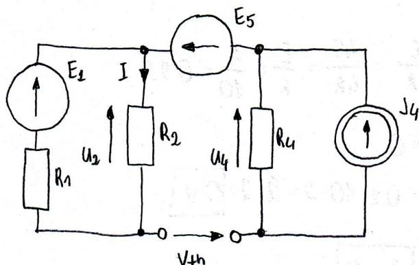
$$I = \frac{E_1}{R_1 + R_2} \quad U_2 = I \cdot R_2 = \frac{E_1 \cdot R_2}{R_1 + R_2} = \frac{2 \cdot 2}{1+2} = \frac{6}{3} = 2\ V$$
