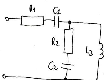
$$R_1 = 10\Omega, R_2 = 5\Omega, X_{C1} = 20\Omega, X_{C2} = 10\Omega, X_{L3} = 20\Omega$$
