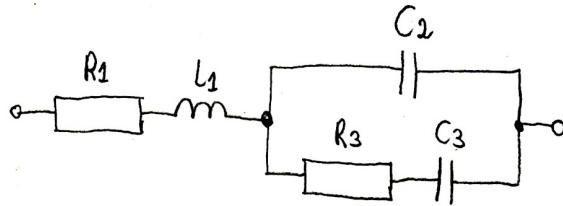
$$R_1 = 10\Omega, R_3 = 20\Omega, L_1 = 50mH$$
