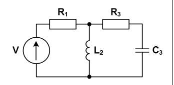
4. The circuit as shown in the figure has been protected by a 6 A overcurrent circuit breaker. Check that it will ensure continuous operation of this circuit when supplied with a sine wave voltage of 24 V rms.
