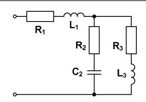
2. Calculate **meter readings** in the circuit shown in the figure.
