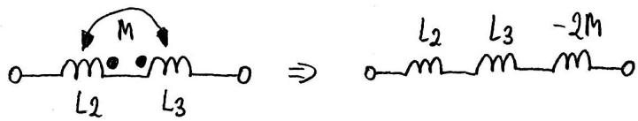
$$Z = R_1 + R_2 + jX_{L2} + jX_{L3} - j2X_M + R_3 - jX_{C_4} + jX_{L4} = 15 + 30 + j10 + j40 - j20 + 15 - j20 + j30 = (60 + j40) \Omega$$
