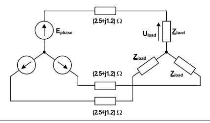
4. The line-to-line voltage of a balanced 3-phase distribution line is  $U_{LL} = 380 \text{ V rms}$ . The load impedance per phase is  $\underline{Z}_L = (30+j20) \Omega$ . Calculate the line currents and the active power of the load for the following configurations of load impedance: a) a wye-connected system, b) a delta-connected system.
