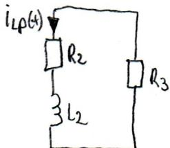
$i_{Lp}(t) = 0 \leftarrow$  because there is no voltage source in the circuit
