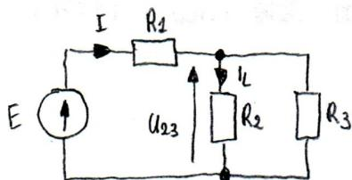
$$I = \frac{E}{R_1 + \frac{R_2 \cdot R_3}{R_2 + R_3}} = \frac{80}{120 + \frac{50 \cdot 200}{50 + 200}} = \frac{80}{120 + 40} = \frac{80}{160} = 0.5 \text{ A}$$
