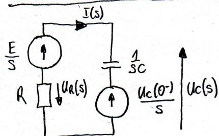
$$I(s) = \frac{\frac{E}{s} - \frac{u_C(0^-)}{s}}{R + \frac{1}{sC}} = \frac{E - u_C(0^-)}{s(R + \frac{1}{sC})} = \frac{E - \frac{2}{3}E}{sR + \frac{1}{sC}} = \frac{\frac{1}{3}E}{s + \frac{1}{RC}} = \boxed{\frac{E}{3R(s + \frac{1}{RC})}}$$
