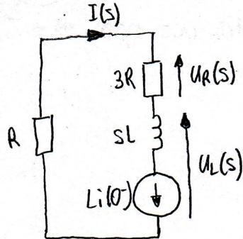
\* next, we solve the circuit equations algebraically in the complex frequency domain using already known methods: Ohm's Law, KVL, KCL, loop-current method, node-voltage method, etc.
