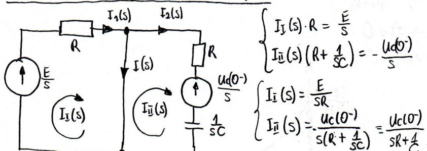
$$I(s) = I_I(s) - I_{II}(s) = \frac{E}{Rs} + \frac{u_C(0^-)}{sR + \frac{1}{sC}} = \frac{E}{Rs} + \frac{E}{R(s + \frac{1}{RC})}$$
