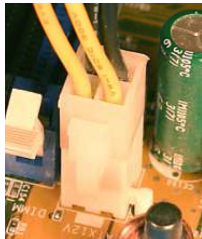
4-pin ATX 12 V
