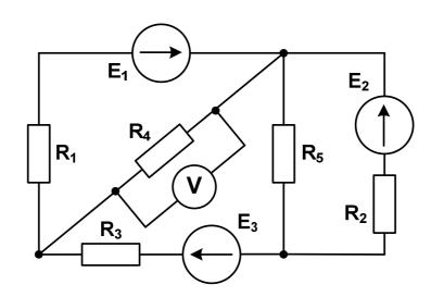
2. Write the equations according to the **Node-Voltage Method** for the circuits shown in the figures.
