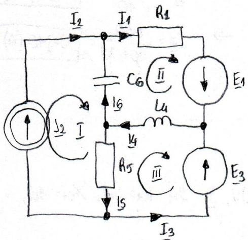
$$\begin{cases} \underline{I_I} = \underline{J_2} = 10A \\ \underline{I_{II}}(R_1 + jX_{L4} - jX_{C6}) - (-jX_{C6}) \cdot \underline{I_I} - (jX_{L4}) \cdot \underline{I_{III}} = E_1 \\ \underline{I_{III}}(R_5 + jX_{L4}) - \underline{I_I}(R_5) - \underline{I_{II}}(jX_{L4}) = -E_3 \end{cases}$$
