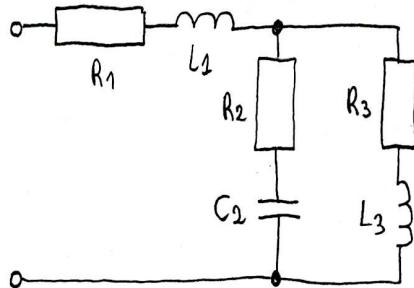
$$R_1 = 10\Omega, R_2 = 5\Omega, R_3 = 15\Omega, L_1 = 50\text{mH}, L_3 = 200\text{mH}, C_2 = 1\text{mF}, \omega = 100 \frac{\text{rad}}{\text{s}}$$
