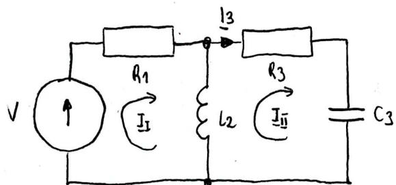
$$\begin{cases} \underline{I}_1(R_1 + jX_{L2}) - \underline{I}_{II}(jX_{L2}) = V \\ -\underline{I}_1(jX_{L2}) + \underline{I}_{II}(R_3 + jX_{L2} - jX_{C3}) = 0 \end{cases}$$
