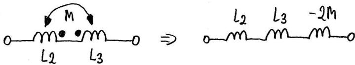
$$Z = R_1 + R_2 + jX_{L2} + jX_{L3} - j2X_M + R_3 - jX_{C4} + jX_{L4} = 15 + 30 + j10 + j40 - j20 + 15 - j20 + j30 = (60 + j40) \Omega$$
