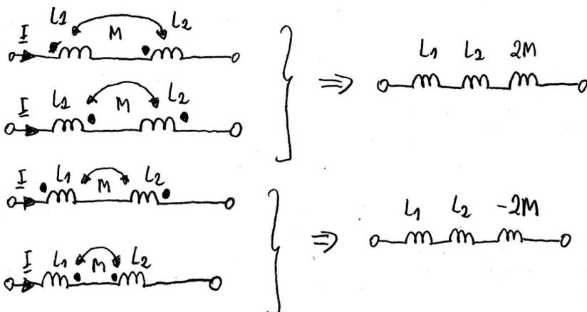
\* if all the flux in one coil reaches the other coil, then we have 100% coupling and  $k=1$
