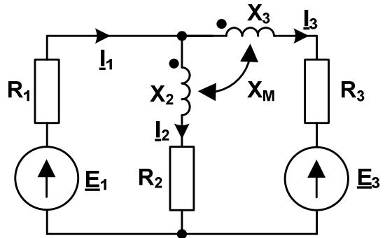
4. What should be the power of the resistor  $R_1$  so that it is not damaged during operation in the circuit shown in the figure.
