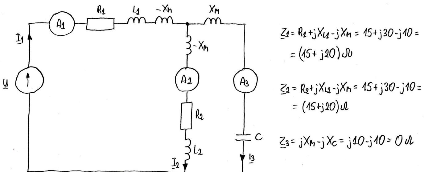
because  $Z_3 = 0 \Omega$  then  $I_{A2} = 0 A$  and  $\underline{I_1} = \underline{I_3}$ ,  $I_{A1} = I_{A3}$   $Z_{eq} = Z_1 = (15 + j20) \Omega$
