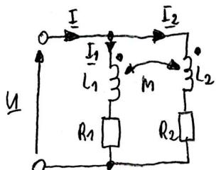
$$\left\{ \begin{array}{l} \underline{I} = \underline{I}_1 + \underline{I}_2 \\ \underline{U} = R_1 \underline{I}_1 + j\omega L_1 \underline{I}_1 + j\omega M \underline{I}_2 \\ \underline{U} = R_2 \underline{I}_2 + j\omega L_2 \underline{I}_2 + j\omega M \underline{I}_1 \end{array} \right.$$
