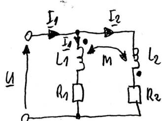
$$\left\{ \begin{array}{l} \underline{I} = \underline{I}_1 + \underline{I}_2 \\ \underline{U} = R_1 \underline{I}_1 + j\omega L_1 \underline{I}_1 - j\omega M \underline{I}_2 \\ \underline{U} = R_2 \underline{I}_2 + j\omega L_2 \underline{I}_2 - j\omega M \underline{I}_1 \end{array} \right.$$
