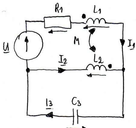
$$\left\{ \begin{array}{l} \underline{I}_1 + \underline{I}_2 = \underline{I}_3 \quad (1) \\ \underline{U} = R_1 \underline{I}_1 + jX_{L_1} \underline{I}_1 - jX_M \underline{I}_2 - jX_{L_2} \underline{I}_2 - (-jX_M \underline{I}_3) \quad (2) \\ 0 = jX_{L_2} \underline{I}_2 - jX_M \underline{I}_1 + (-jX_C \underline{I}_3) \quad (3) \end{array} \right.$$
