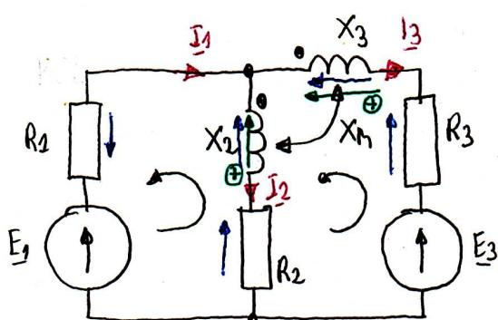
$$\text{KCL: } \underline{I}_1 - \underline{I}_2 - \underline{I}_3 = 0$$
