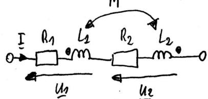
$$\underline{U}_1 = R_1 \underline{I} + j\omega L_1 \underline{I} - j\omega M \underline{I}$$
