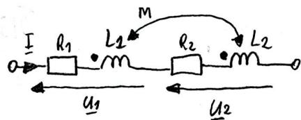
$$\underline{U}_1 = R_1 \underline{I} + j\omega L_1 \underline{I} + j\omega M \underline{I}$$
