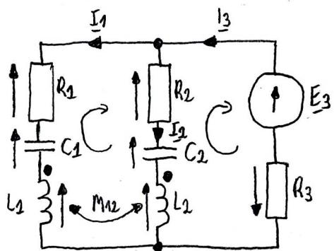
$$\text{KCL} \rightarrow \underline{I_1} + \underline{I_2} = \underline{I_3}$$
