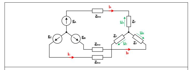
3. In the 3-phase balanced Y-Y system, the load voltage is  $U_{load} = 400 \angle -20^{\circ} \text{ V rms}$ , the line impedance is  $(2.5+j1.2) \Omega$ , and the source voltage is  $E_{phase} = 440 \text{ V rms}$ . Find the load impedance, its power, and the value of supplying current.
