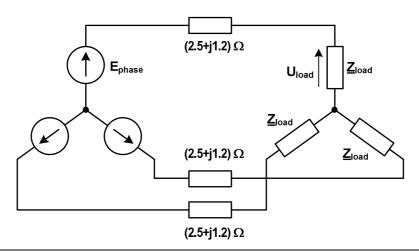
4. The line-to-line voltage of a balanced 3-phase distribution line is  $U_{LL} = 380 \text{ V rms}$ . The load impedance per phase is  $\underline{Z}_L = (30+j20) \Omega$ . Calculate the line currents and the active power of the load for the following configurations of load impedance: a) a wye-connected system, b) a delta-connected system.
