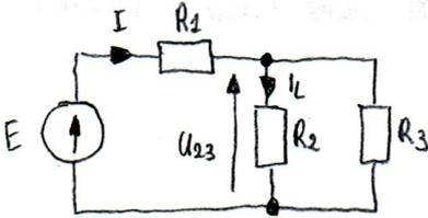
$$I = \frac{E}{R_1 + \frac{R_2 \cdot R_3}{R_2 + R_3}} = \frac{80}{120 + \frac{50 \cdot 200}{50 + 200}} = \frac{80}{120 + 40} = \frac{80}{160} = 0.5 \text{ A}$$
