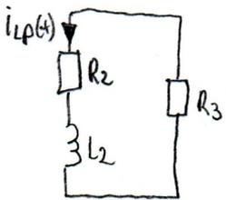
$i_{LP}(t) = 0$  ← because there is no voltage source in the circuit
